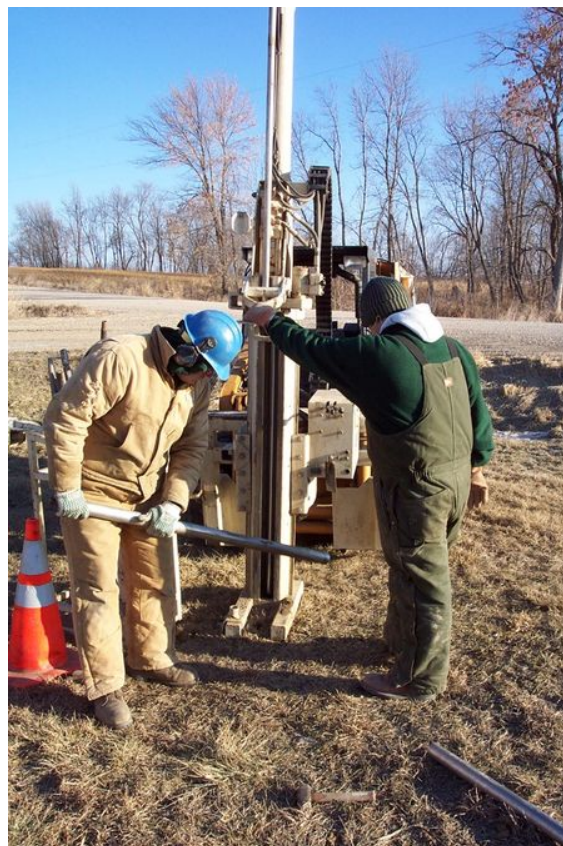
Example of direct push technology used to collect a soil sample.
