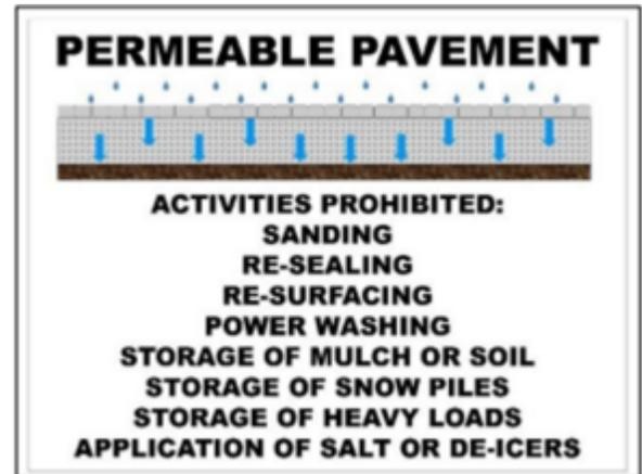
Example sign to be placed adjacent to permeable pavements. Source: North Carolina Department of Environmental Quality (<https://files.nc.gov/ncdeq/Energy%20Mineral%20and%20Land%20Resources/Stormwater/BMP%20Manual/C-5%20%20Permeable%20Pavement%2004-06-17.pdf>).
