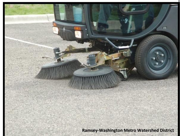
\*A vacuum sweeper is a piece of equipment that removes sediment and other types of debris from the spaces on the pavement surface. This must be done twice a year to effectively help keep the pervious pavement free of debris so that water is able to soak into the ground as designed.
