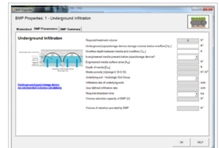
Screenshot from MIDS calculator showing user inputs needed for underground infiltration. The link located below the image is to a page that allows the user to make necessary calculations for V_p and A_M .
