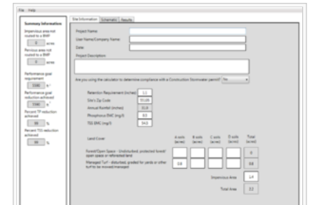
Screen shot of the Site Information tab for underground infiltration. In this example, the user has entered a ZIP code and acres of pervious and impervious surfaces. Note also the user must indicate whether or not the calculator is being used to determine compliance with the Construction Stormwater permit. See Step 2.
