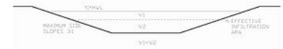
Schematic showing the effective infiltration area for side slopes less than 3H:1V.
