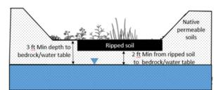
Schematic illustrating separation distance from bottom of infiltration BMP to water table or top of bedrock. This diagram includes a modified subsoil zone in which the subsoil has been ripped to alleviate compaction.
