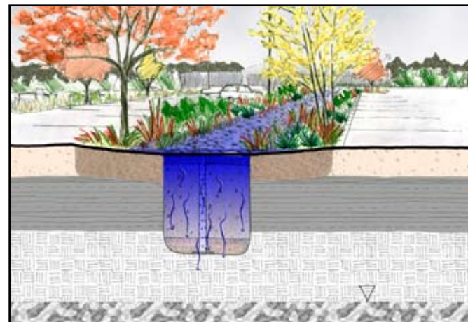
Duration of Storm Event - Storage & filtration/infiltration
