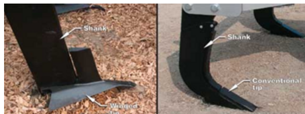
Photos of wing tip and conventional tip subsoilers (Kees, 2008).
