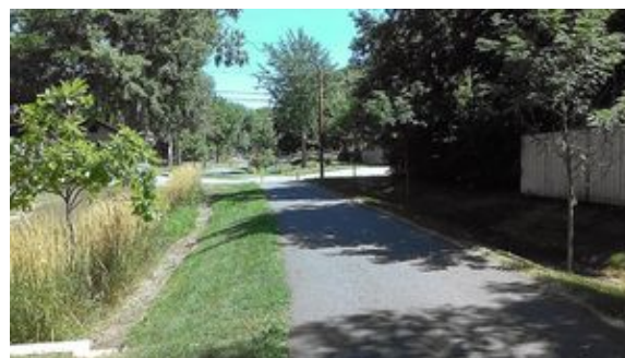
The vegetated filter strip in this photo is pretreatment for a bioswale. Photo courtesy of Alisha Goldstein, U.S. EPA.
