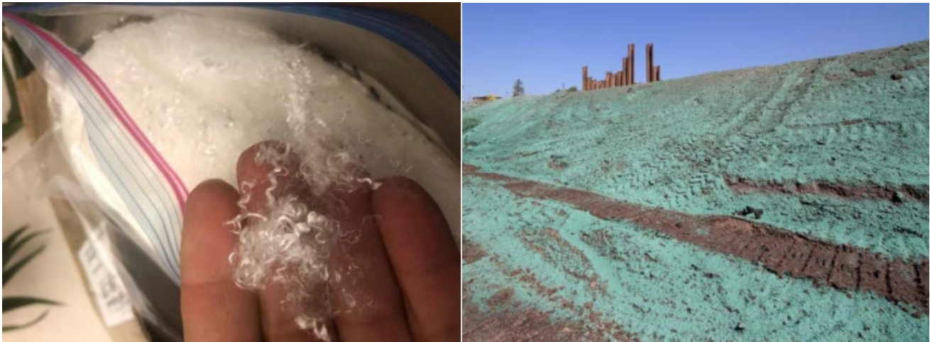
Synthetic fibers (left) and Malachite Green (right) used in hydraulic applications. Image courtesy of MnDOT and MNDNR.
