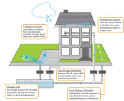
Schematic illustrating the basic concepts for a harvest and use-reuse system. Stormwater or rainwater is stored in a cistern or pond and delivered outdoors or indoors through a distribution system.
