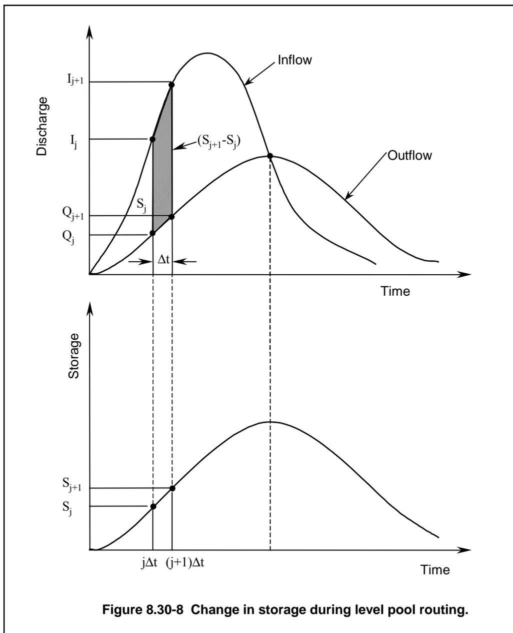
**Figure 8.30-8 Change in storage during level pool routing.**
