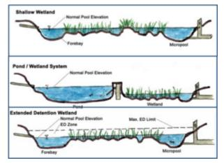
The three major stormwater wetland types include shallow wetlands, a pond/wetland system, and an extended detention wetland
