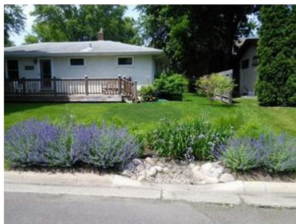
A rain garden in a residential development. Photo courtesy of Katherine Sullivan.
