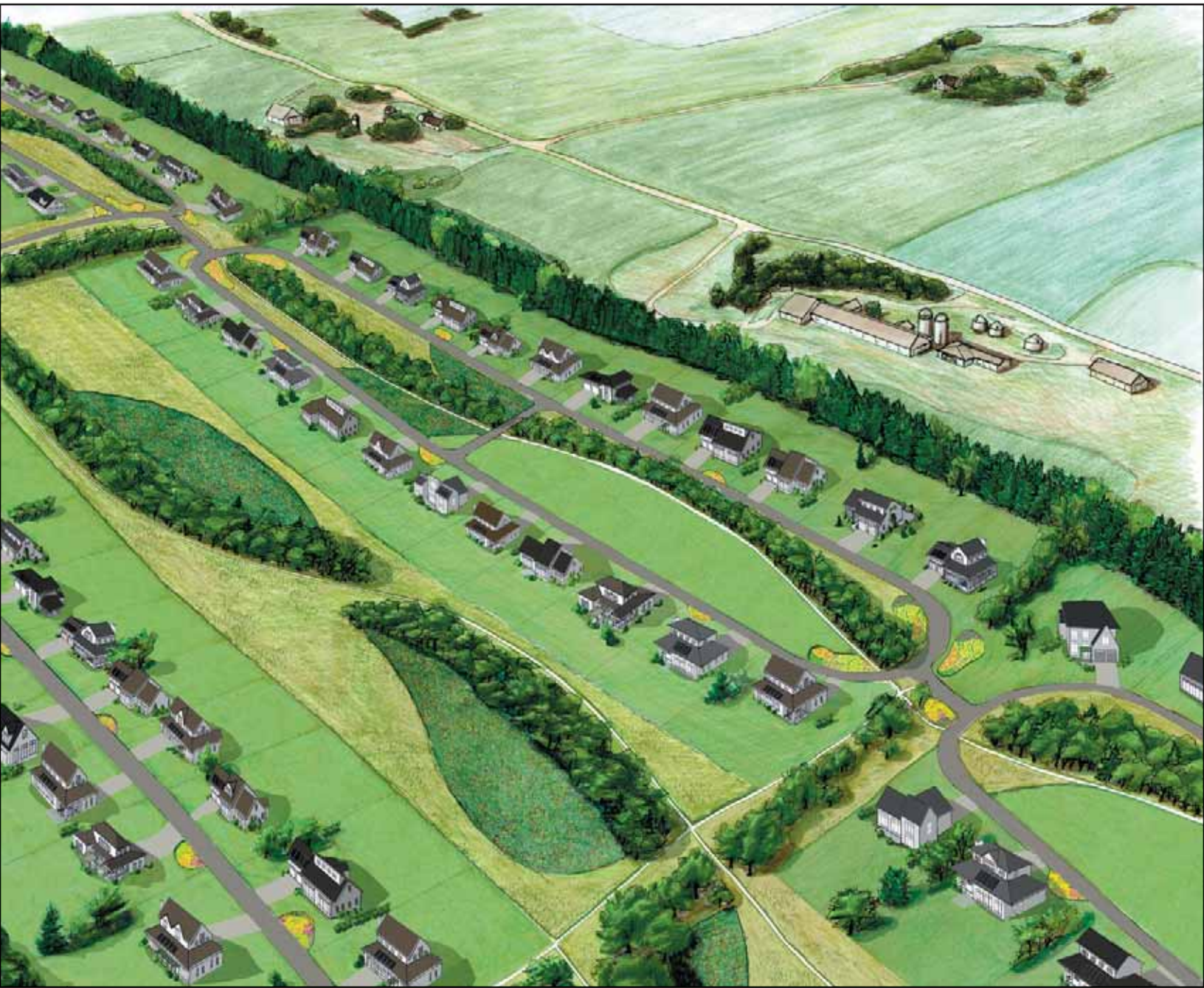
This prototypic design for a property in Hanover, Minnesota, used the conservation design process for neighborhood layout. The plan features 50 percent open space with green space adjacent to every back yard, a trail system, habitat creation, distinct neighborhoods, and a natural stormwater management system.
