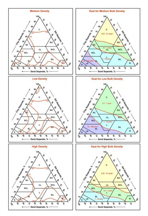
Note: Estimate saturated hydraulic conductivity (K<sub>sat</sub>) from soil texture by first selecting the bulk density class of medium, low or high. Then use the corresponding textural triangle to select the range of saturated hydraulic conductivity in mms-1.
