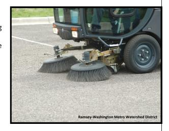
\*A vacuum sweeper is a piece of equipment that removes sediment and other types of debris from the spaces on the pavement surface. This must be done twice a year to effectively help keep the pervious pavement free of debris so that water is able to soak into the ground as designed.
